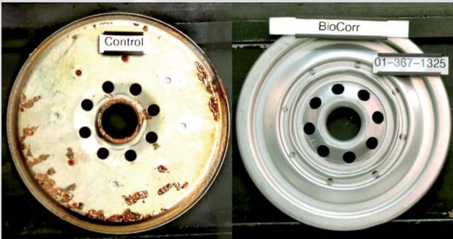
The pictures shows a test ran in our humidity cabinet. These parts were run at 50°C and >95% humidity for 360 hours..
