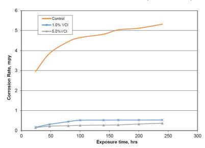
Corrosion behavior of steel pipes in boiling chloride water solution (200 ppm). Corrosion rate (mpy) of untreated control (orange) versus samples treated with 1% CorroLogic® CUI High-Temp Inhibitor (blue) and 5% CorroLogic® High-Temp Inhibitor (gray).
