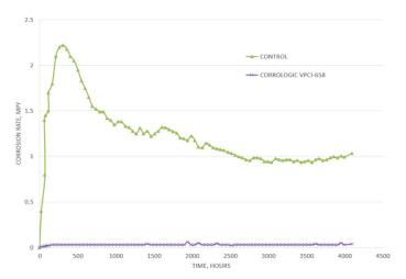
$\ensuremath{\mathsf{ER}}$  (electrical resistance) probe corrosion readings over 4000 hours of testing.
