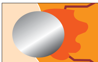
Cracking and spalling will ultimately occur.
