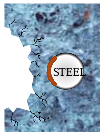
Remove spalled concrete from deteriorating structure.
