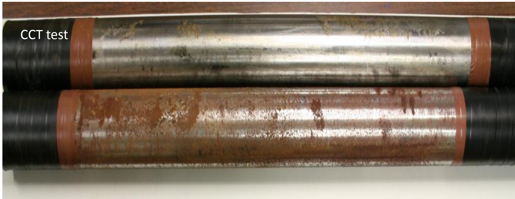
Comparison of Corrosion behavior of steel Pipes, Day 30
