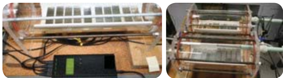
FIGURE 2. Test setup for the controlled humidity corrosion tests on UNS G102000 steel and galvanized steel samples. ER probes were in environments with 10% VCI or nitrogen blanketing at 10 psi applied pressure.
