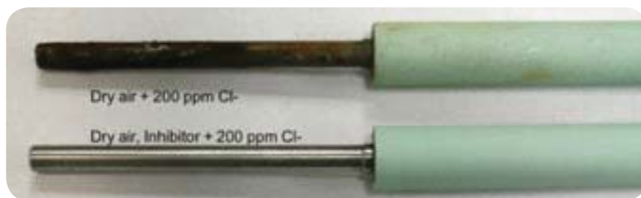
FIGURE 4. ER probes after 4,464 h exposure; top probe exposed to dry air, lower probe protected with inhibitor.
