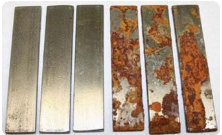
FIGURE 7. Comparison of UNS G10200 steel samples after 155 days: (left) inhibitor still providing protection, (right) samples exposed to dry air in test chamber.
