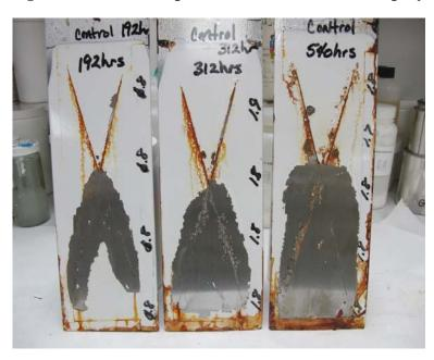
The result in Figure 7 presents the poor performance of an acrylic water-based paint with no inhibitors other than for flash rust. The paint failed  $\leq 192$ hrs in the salt chamber (*Failure*  $\geq 3mm$  creep from scribe). The salt vapors were able to quickly penetrate the film's barrier which leads to blistering and loss of adhesion causing the underlying substrate to corrode (see figure 8).
