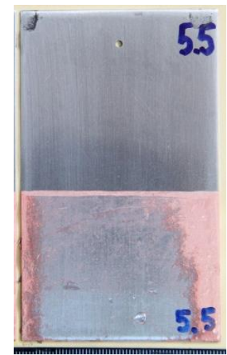
FAIL, 70% of surface still covered with RP
