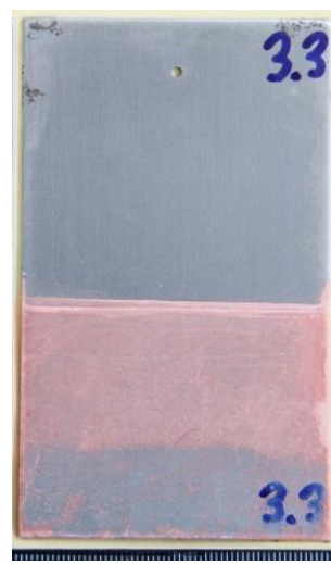
FAIL, 30% of surface still covered with RP
