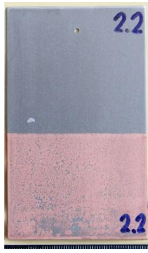
FAIL, 5% of surface still covered with RP
