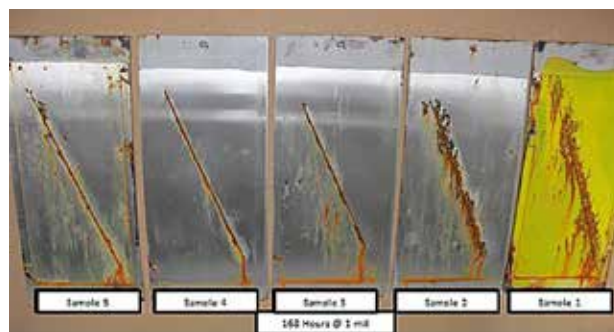
FIGURE 2 Control panels failed after 168 h in the salt fog cabinet.
