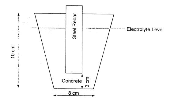
Figure 1. Concrete specimen used in this study.
