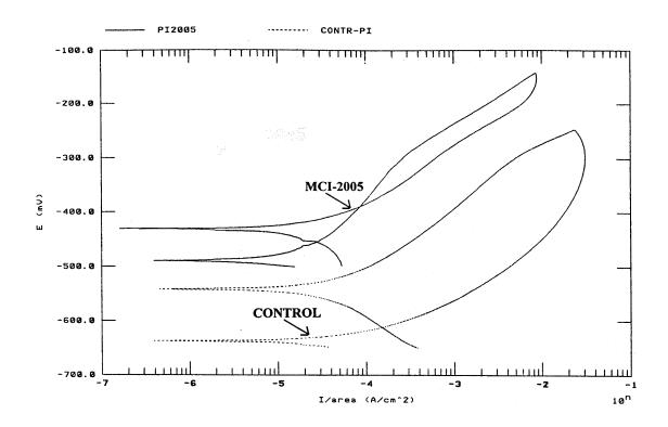
Figure 3. Cyclic polarization plots of solutions with and without MCI-2005.
