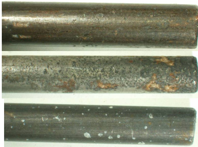
Figure 3 Reinforcing steel after corrosion testing from specimens 056 - reference ones
