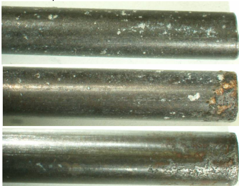
Figure 4 Reinforcing steel after corrosion testing from specimens 057 - with MCI 2005
