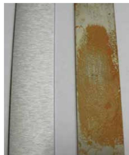
Immersion of carbon steel in IRB treated water (L) vs. untreated water (R).
