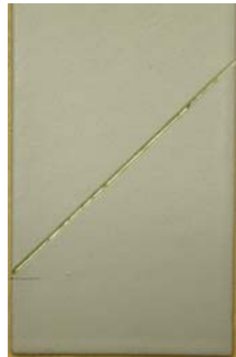
FIGURE 11 - Coated and scribed steel coupon after 9 months exposure in control test vessel, showing very mild corrosion in the scribes.
