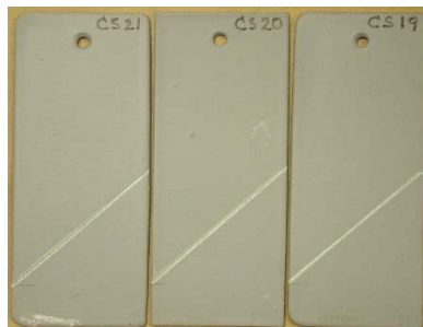
FIGURE 12 - Coated and scribed steel coupons after 9 months exposure to VCI A showing no corrosion in the scribes
