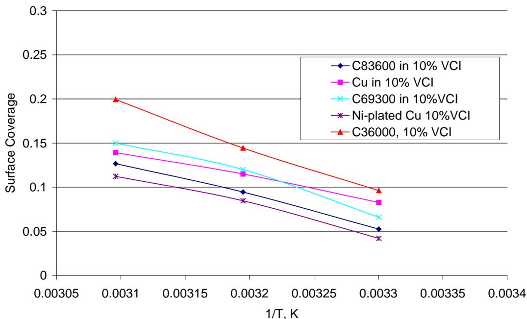
Figure 6: Langmuir adsorption isotherm showing the relationship between surface coverage, Inhibitor-A and temperature for different alloys.
