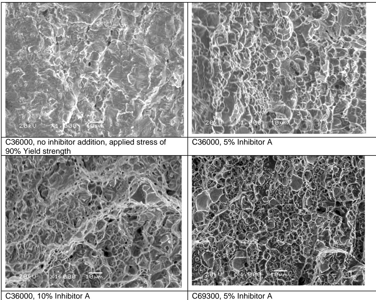
Figure 5: SEM fractographs of the fracture surface for C-ring samples of C36000 after SCC tests in different solutions.
