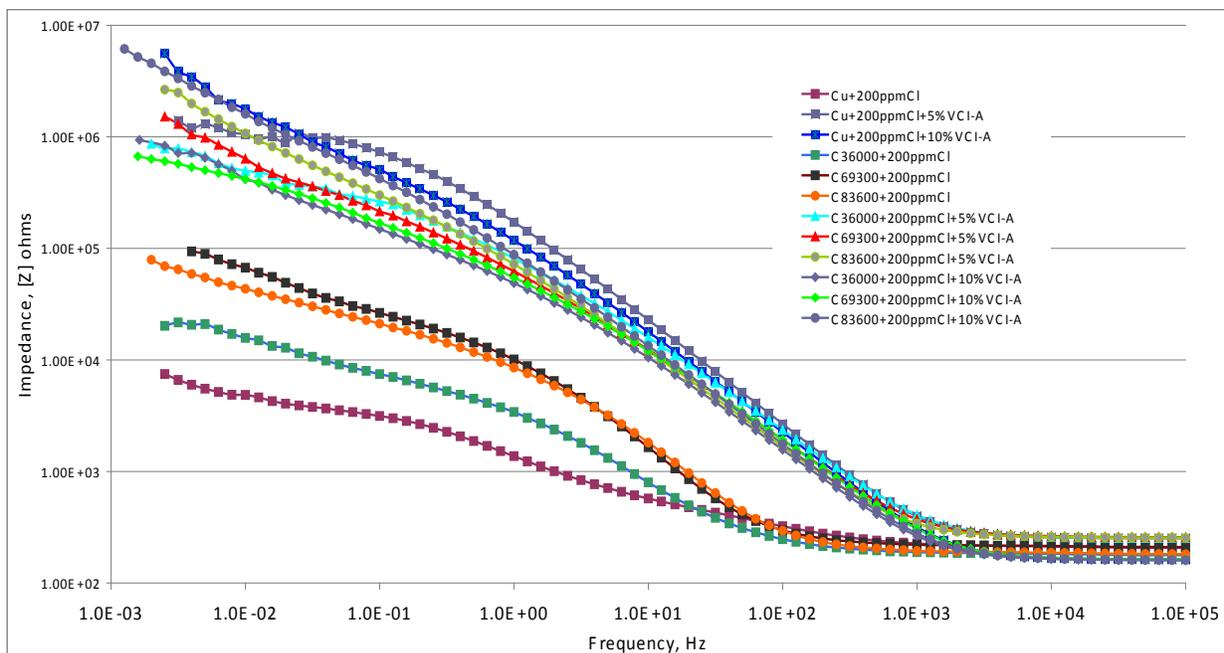
Figure 3: Electrochemical impedance spectroscopy Bode plots for Cu, C36000, C69300 and C83600 brass in different Inhibitor-A concentrations.
