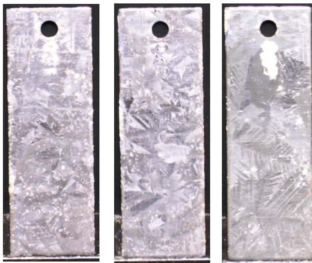
Figure 2. Galvanized Steel Coupons – Formulation 1 @ 170ppm
