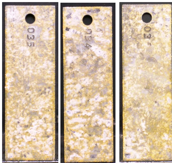
Figure 1. Galvanized Steel Coupons – Control
