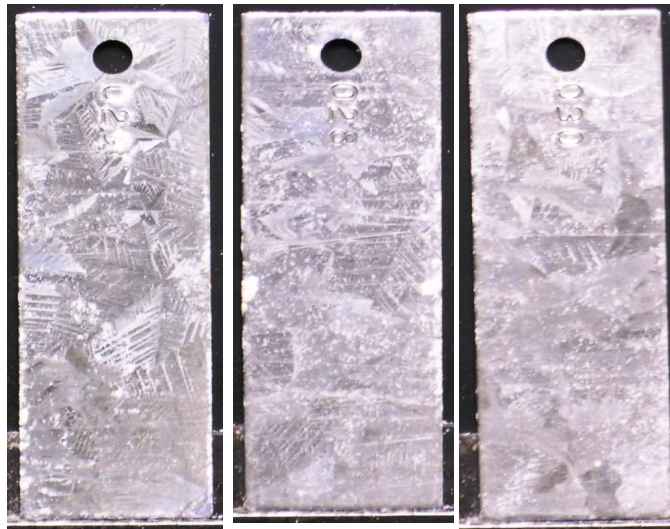
Figure 3. Galvanized Steel Coupons – Formulation 1 + VpCI A @ 170ppm
