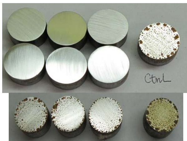
FIGURE 6. Plugs from VIA test of enhanced sugar beet molasses (1g sample) (Top row: sugar beet molasses with 1.5% NH 4 OH, Middle row: sugar beet molasses with 5% monoethanolamine, Bottom row: NH 4 OH only. The right most plugs are from the control)
