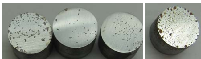
FIGURE 4: Plugs after VIA test on sugar cane molasses as-received (5 g sample) vs Control Plug (Right)
