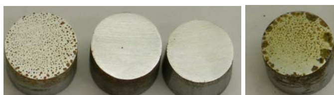
FIGURE 3: Plugs after VIA test on sugar beet molasses as-received (5 g sample) vs Control Plug (Right)
