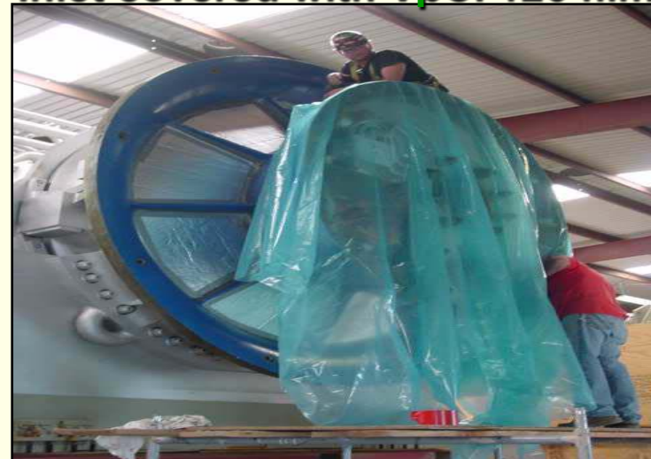
Inlet covered with VpCI 126 film
