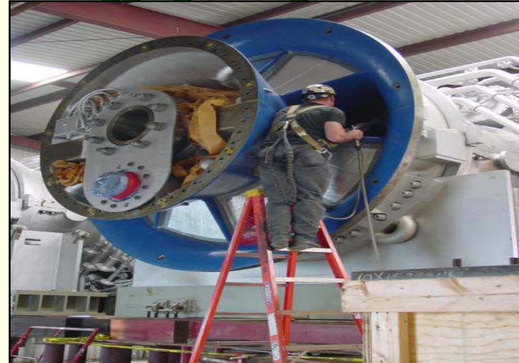
Inlet covered with VpCI 126 film
