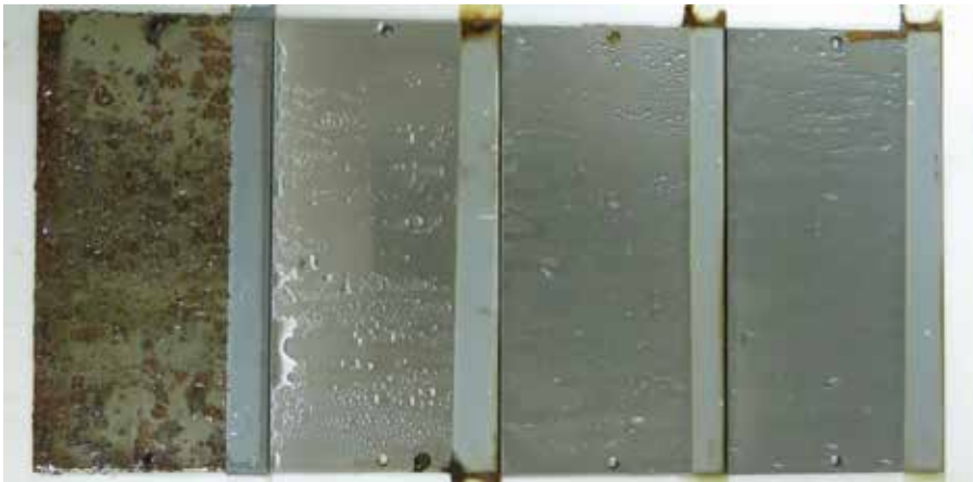
FIGURE 2. ASTM D1735 test results with Product A. The control panel is pictured on the far left.
