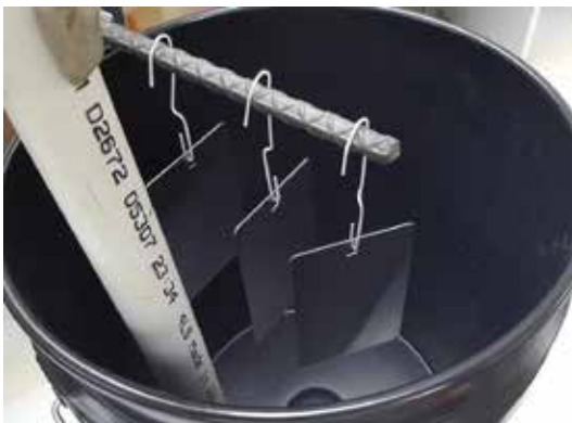
FIGURE 3. Image of the inside of the float coating test vessel. The vessel can accommodate several standard 4- by 12-in test panels (3- by 5-in test panels are pictured above).
