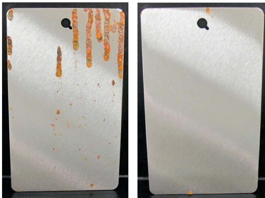
FIGURE 1 Panels at end of accelerated corrosion test; control (left) and sample with VCI-2 (right).
