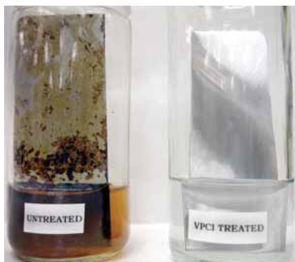
The untreated panel on the left shows extensive corrosion from damaging deposits. The panel on the right, which was treated with a vapor-phase corrosion inhibitor (VPCI), is corrosion-free. VPCIs can greatly extend the life of cooling towers.
