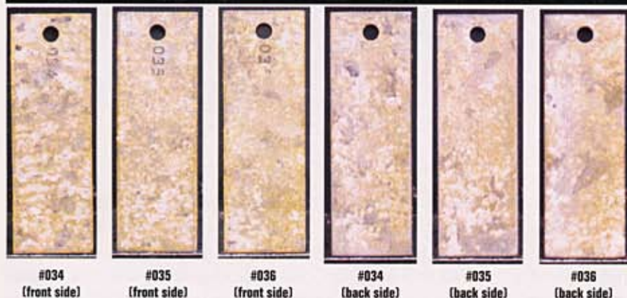
Galvanized steel coupons—control.
