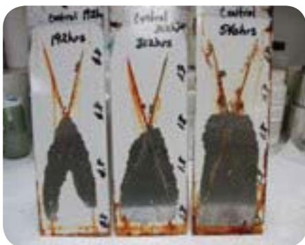
**FIGURE 7.** Control sample, 540 h of continuous salt spray.
