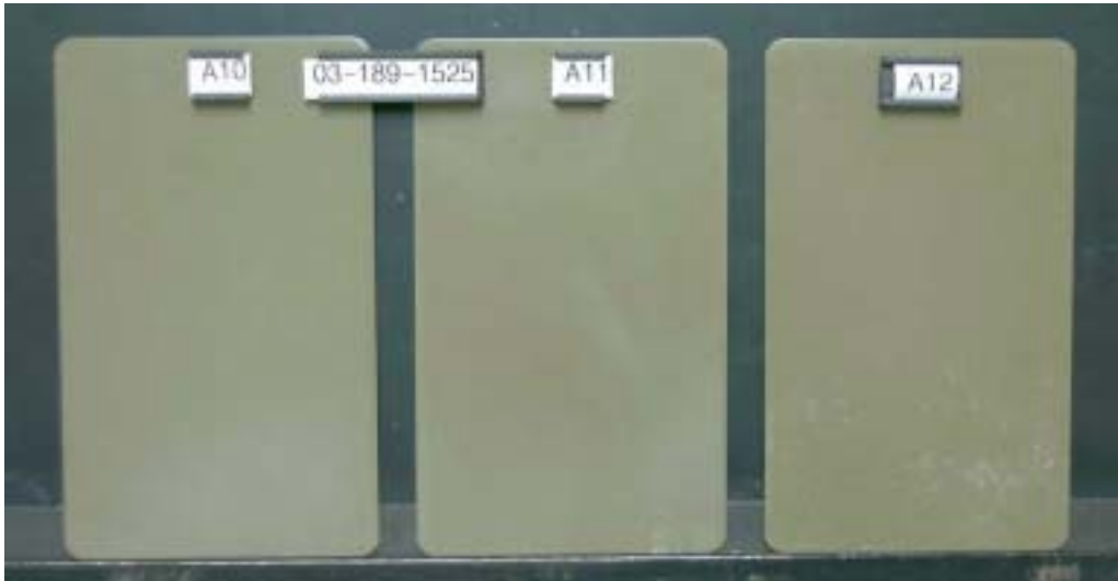
Panels A10, A11, A12 after 80 cycles in GM 9540 P, after cleaning
