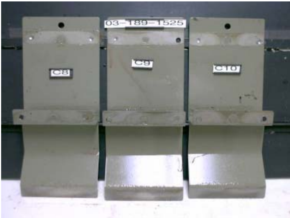
Panels C8, C9, C10 after 40 cycles in GM 9540P
