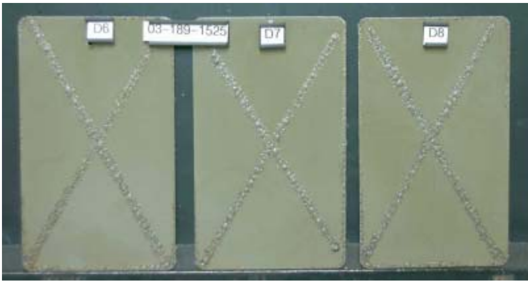
Panels D6, D7, D8 after 80 cycles in GM 9540 P, after cleaning
