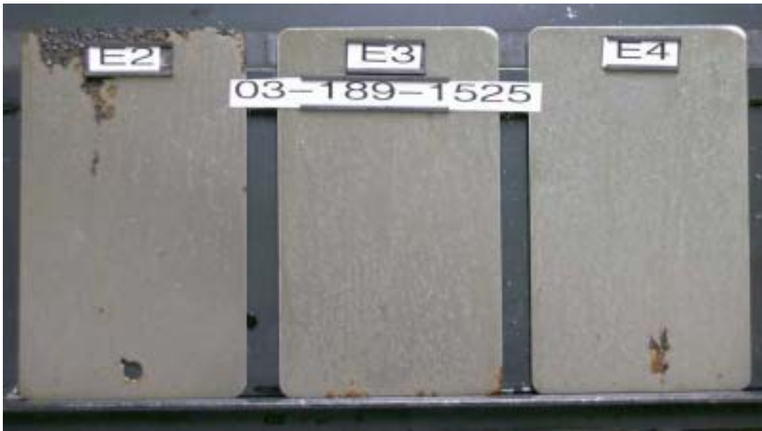
Panels E2, E3, E4 after 40 cycles in GM 9540P
