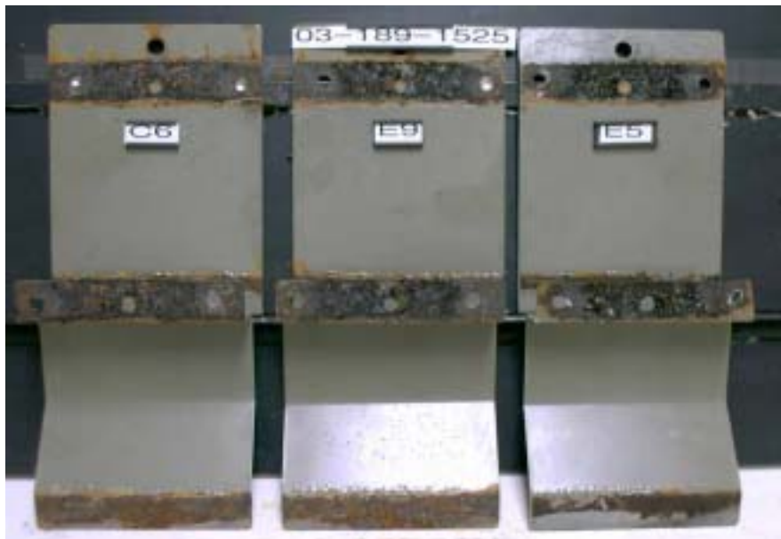
Panels C6, E5, E9 after 40 cycles in GM 9540P
