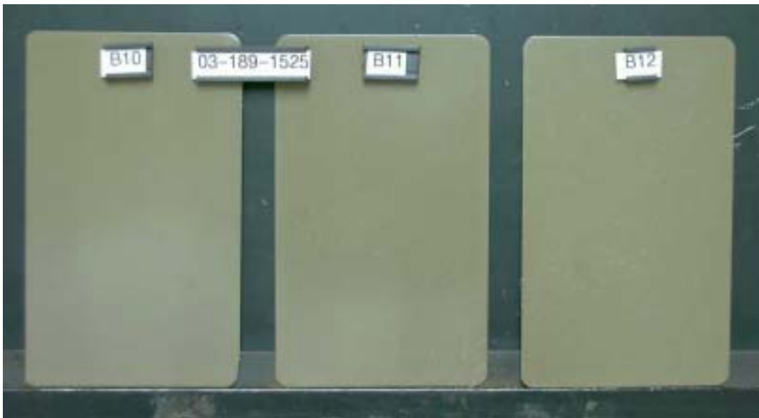
Panels B10, B11, B12 after 80 cycles in GM 9540 P, after cleaning
