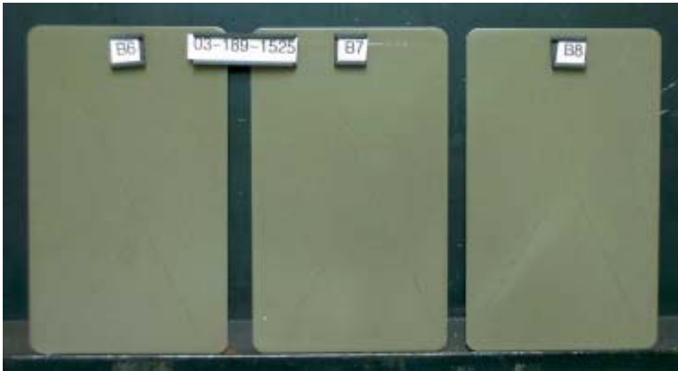
Panels B6, B7, B8 after 80 cycles in GM 9540 P, after cleaning
