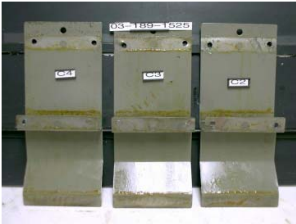
Panels C2, C3, C4 after 40 cycles in GM 9540P
