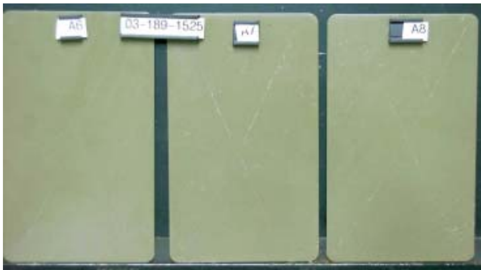
Panels A6, A8, A7 after 80 cycles in GM 9540 P, after cleaning
