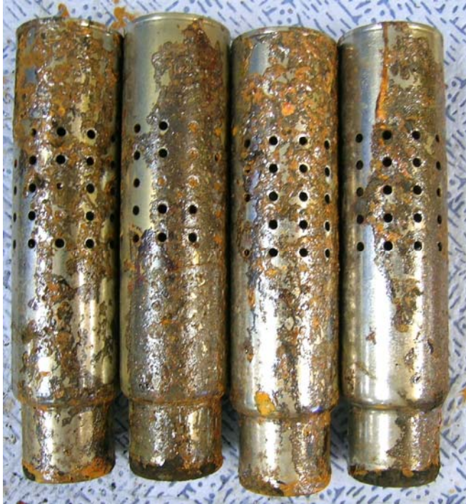
Figure 2: A1, control parts after 1000 hours in ASTM D-1748 humidity.
