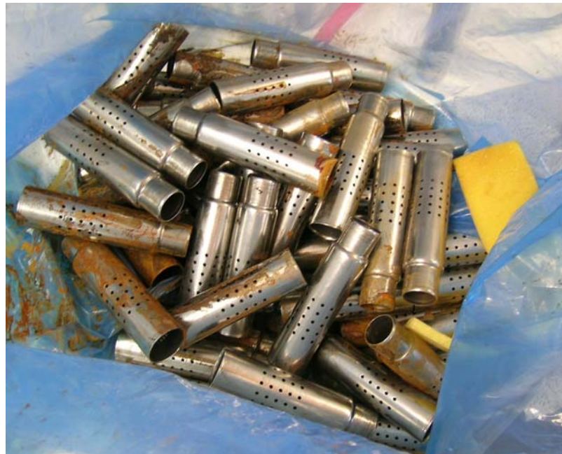
Figure 6: D1, parts packaged in unknown blue film with VpCI-131 foam pad, after 1000 hours in ASTM D-1748 humidity.
