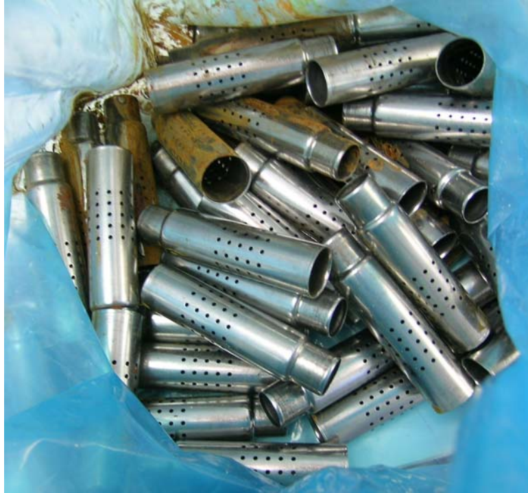
Figure 7: E1, parts packaged in 2-mil VpCI-126 blue film, after 1000 hours in ASTM D-1748 humidity.
