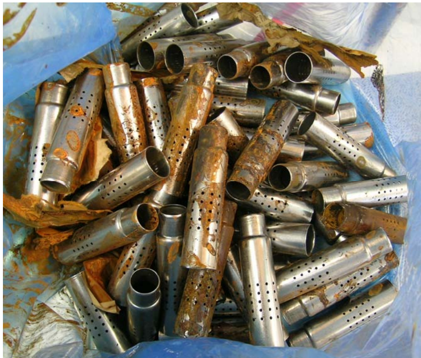
Figure 3: B1, parts packaged in unknown blue film with Armor VCI paper, after 1000 hours in ASTM D-1748 humidity.
