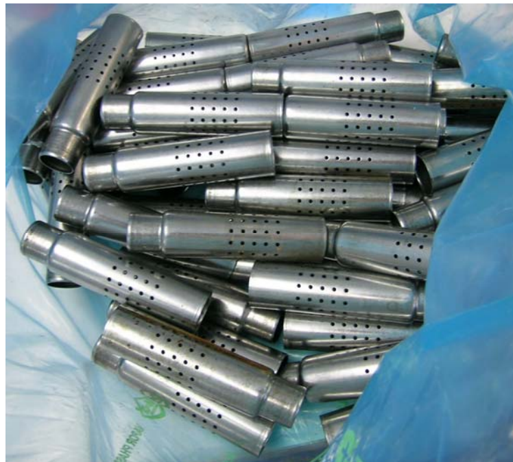
Figure 8: F1, parts packaged in 4-mil VpCI-126 film, after 1000 hours in ASTM D-1748 humidity.
