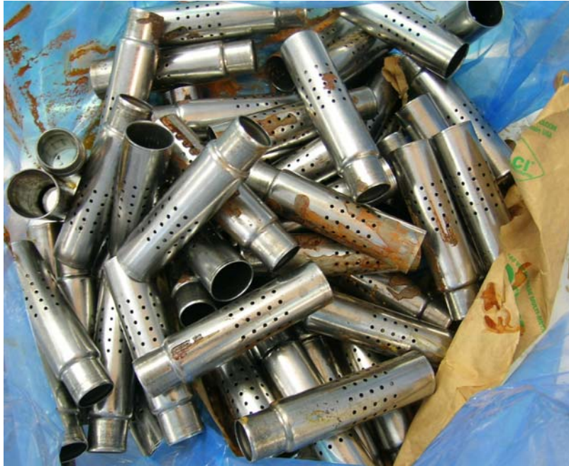
Figure 5: C1, parts packaged in unknown blue film with VpCI-146 paper, after 1000 hours in ASTM D-1748 humidity.
