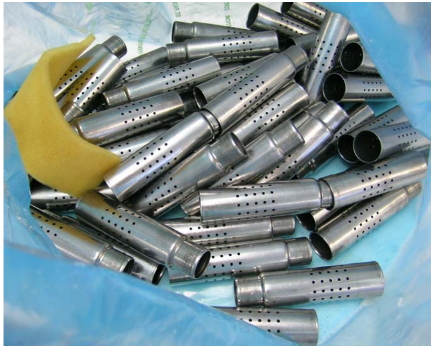
Figure 10: H1, parts packaged in 4-mil VpCI-126 and VpCI-131 foam, after 1000 hours in ASTM D-1748 humidity
