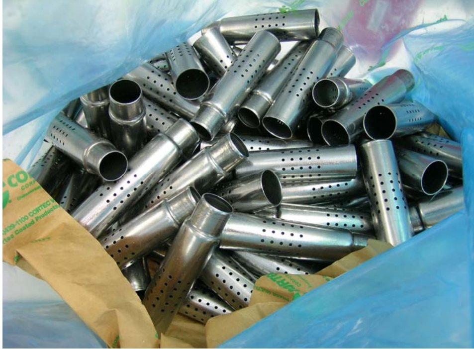
Figure 9: G1, parts packaged in 4-mil VpCI-126 and VpCI-146 paper, after 1000 hours in ASTM D-1748 humidity.
