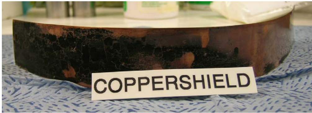
Figure 2: Copper strip dipped in Coppershield (4.5% solution), after 312 hours in ASTM D-1748 humidity cabinet testing.
