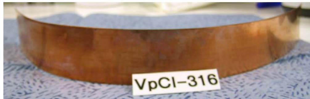
Figure 4: Copper strip dipped in VpCI-316 (5% solution), after 312 hours in ASTM D-1748 humidity cabinet testing.
