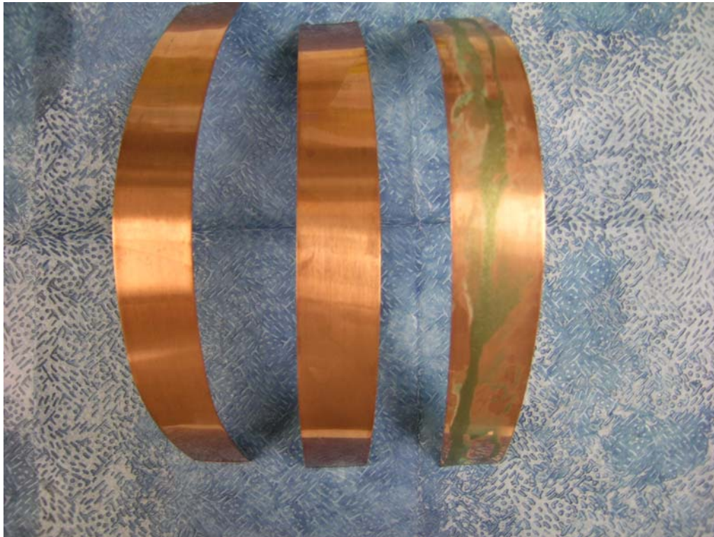
Figure 1: Copper strips, after dipping, prior to testing. From left to right: VpCI-239, VpCI-316, Coppershield.
