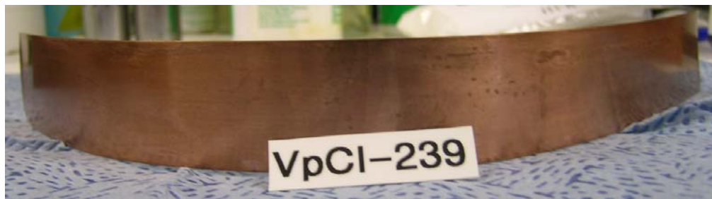
Figure 3: Copper strip dipped in VpCI-239, after 312 hours in ASTM D-1748 humidity cabinet testing.
