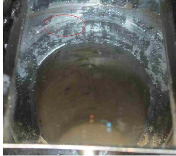
Nov 11: Corrosion formed at the base of the seat pocket. (top of the picture)
