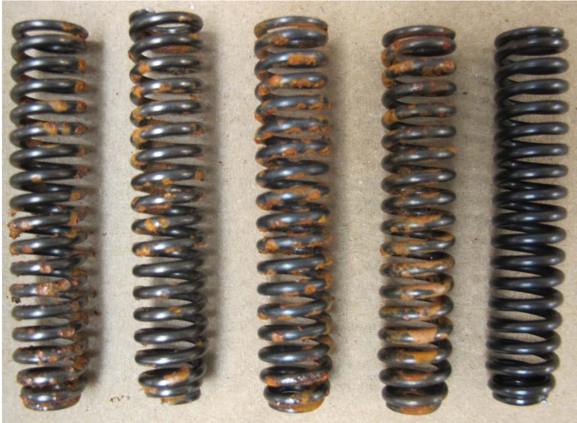
Figure 1: Springs after 72 hours of ASTM D-1748 humidity testing. From L-R: Control, Shaeffer, BioCorr, VpCI-325, EcoLine 3220
