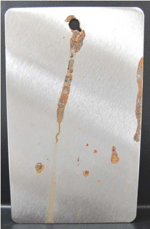
10% Hangsterfer's S-1001 fluid (control)
