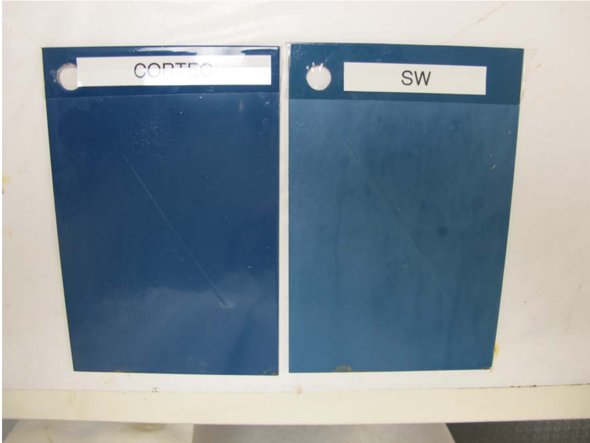
Cold rolled steel panels; ASTM B-117
