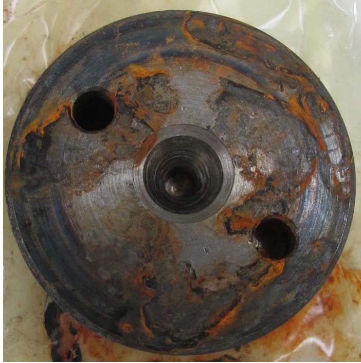
Figure 4: Cimguard 20 + Yellow film wrapped part, after 600 hours of testing.
