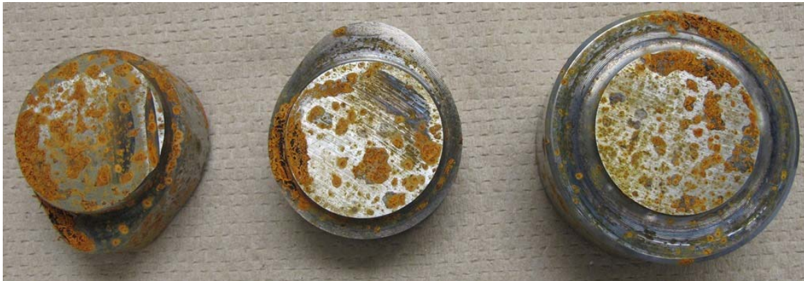
Figure 1: Cinguard 20, BioCorr, and VpCI-329D (left to right) treated parts, after 600 hours of testing. These parts were not wrapped in film for testing.
