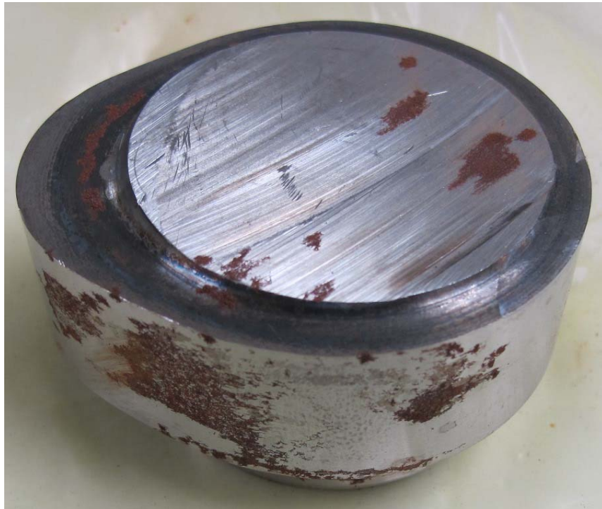
Figure 3: Yellow film wrapped part, after 600 hours of testing.
