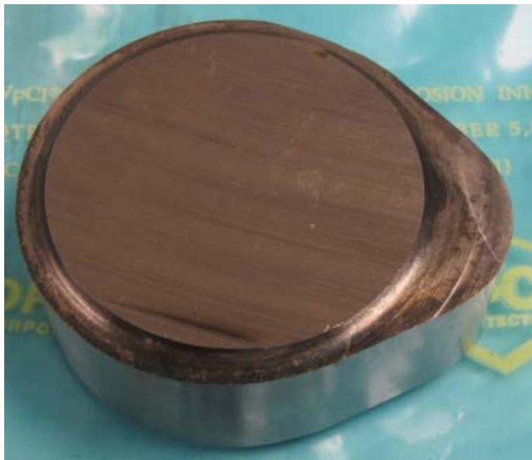
Figure 7: VpCI-329D + VpCI-126 wrapped part, after 600 hours of testing.
