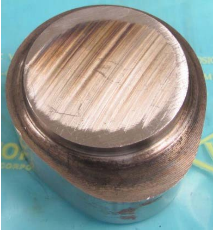
Figure 6: BioCorr + VpCI-126 wrapped part, after 600 hours of testing.
