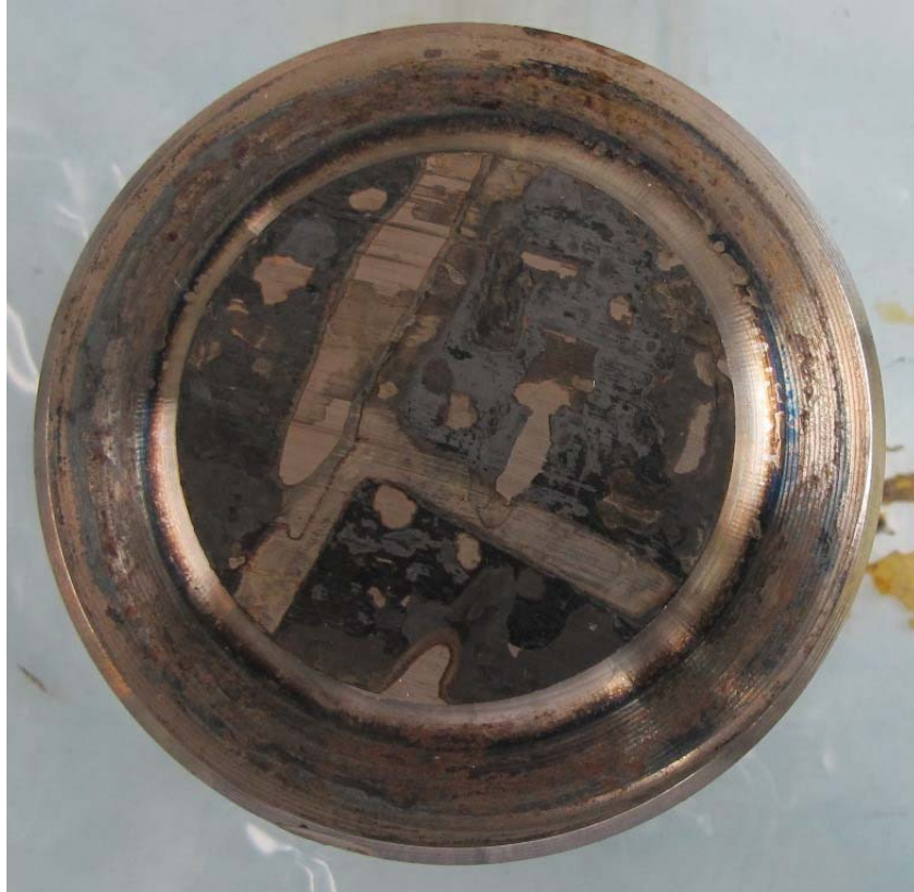
Figure 2: Blue film (current) wrapped part, after 600 hours of testing.
