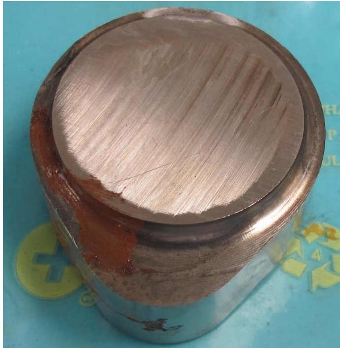
Figure 5: VpCI-126 wrapped part, after 600 hours of testing.
