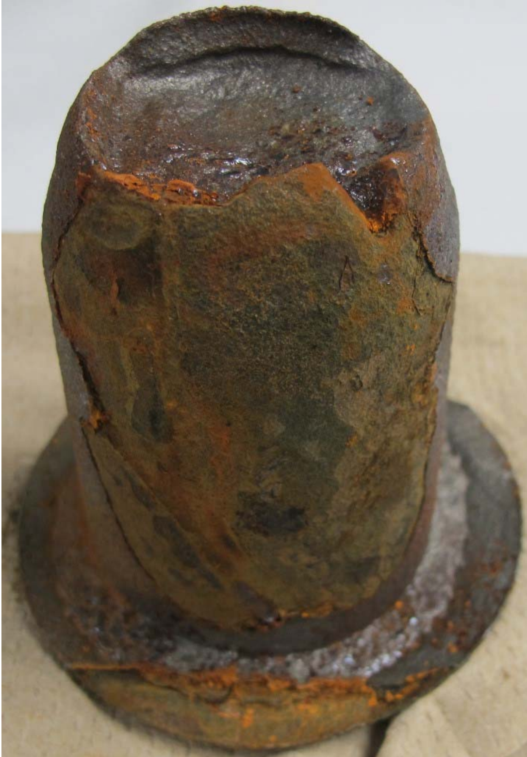
Figure 2: Green film packed part, after 168 hours in ASTM D-1735 testing.
