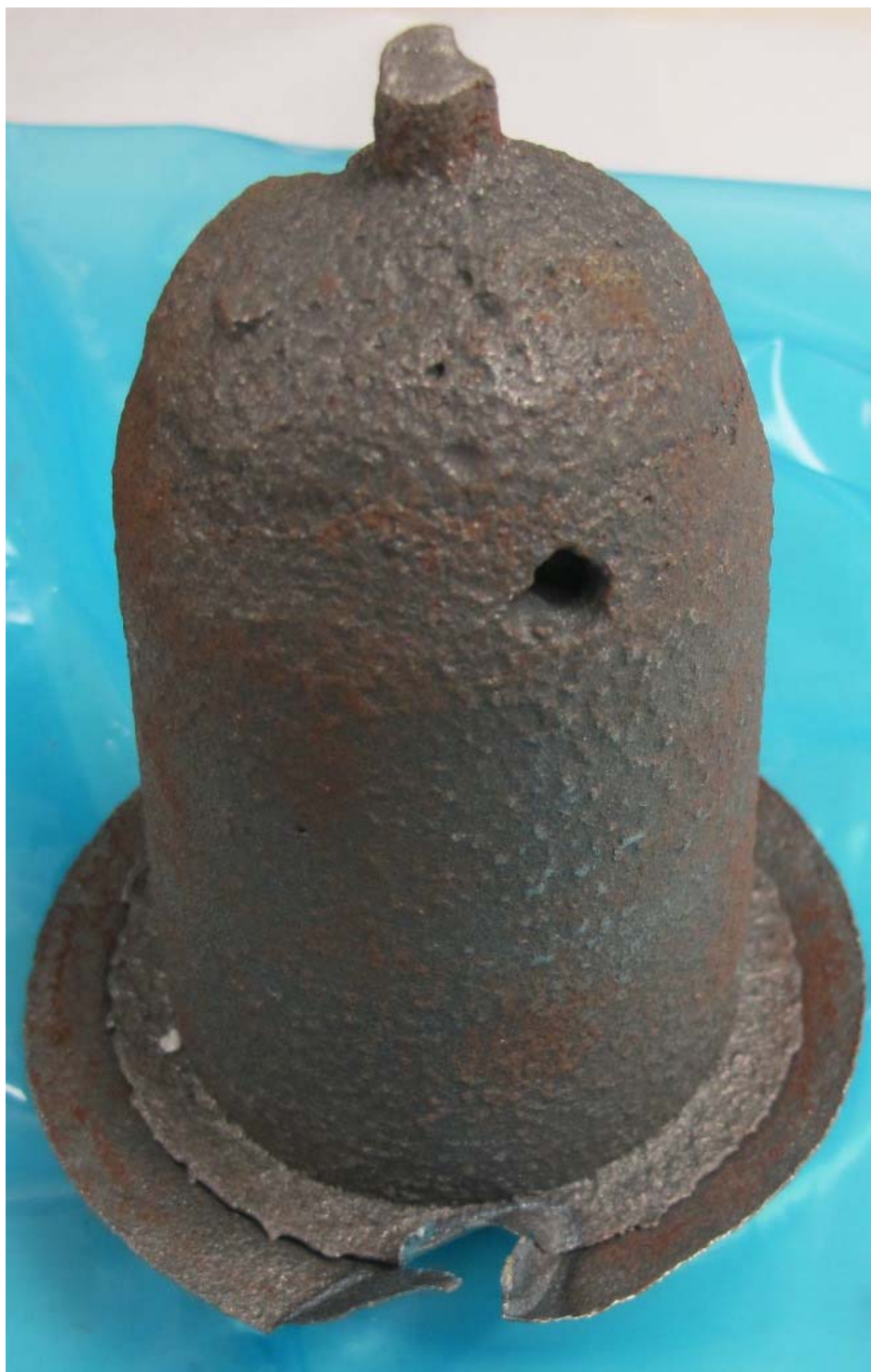
Figure 3: VpCI-126 wrapped part, after 168 hours in ASTM D-1735 testing.
