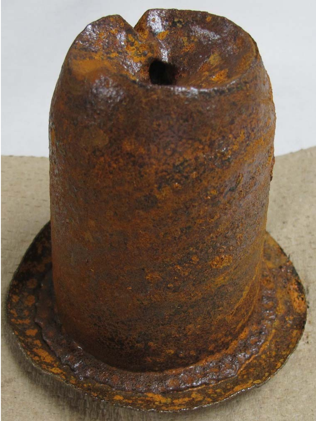
Figure 1: Control part, after 168 hours in ASTM D-1735 testing.
