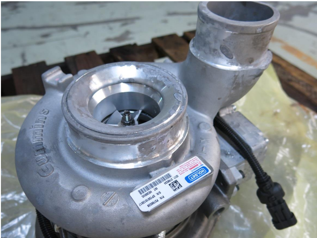
Picture 4: Intake portion of the turbo engine packaged in NT bags after 500 hours. Severe discoloration can be seen at the intake and on the surrounding body of the engine.
