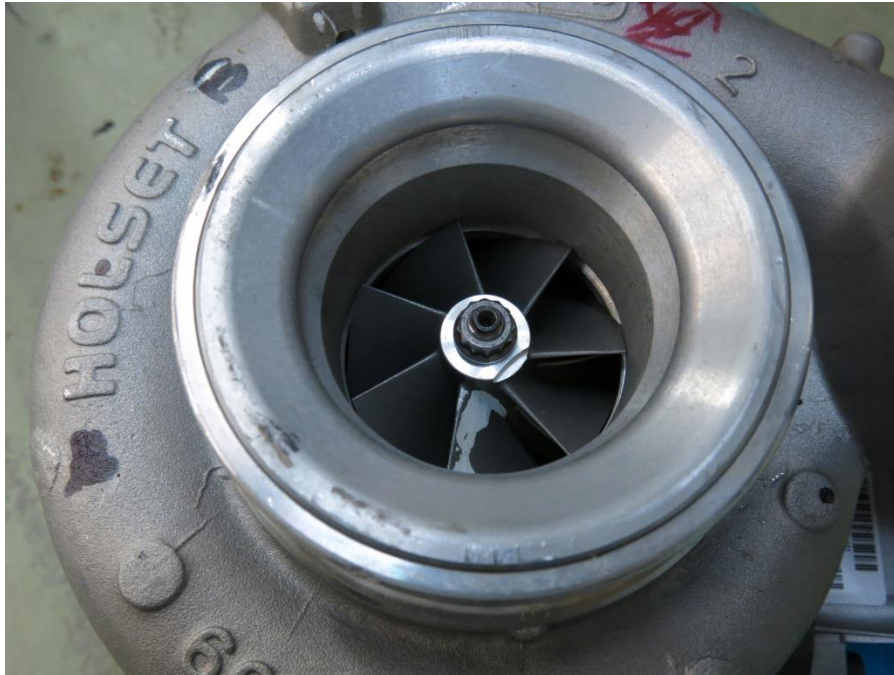
Picture 1: The turbo engine packaged and sealed in VpCI-126 and PE after 300 hours of testing. Little to no discoloration is observed on the intake.
