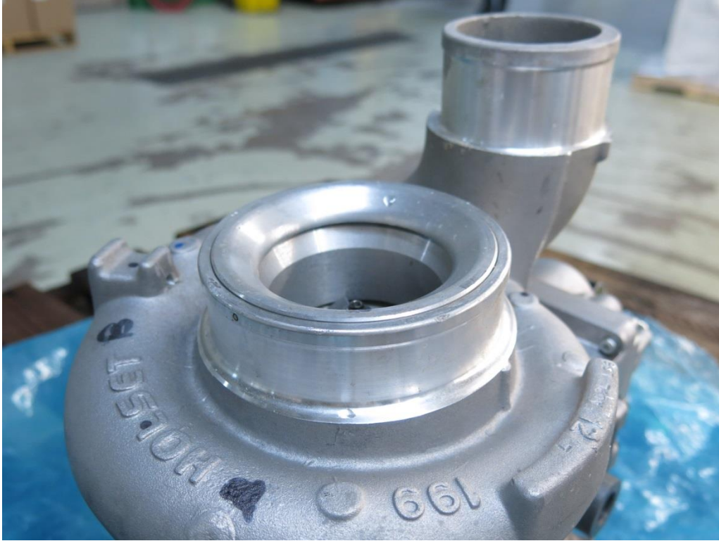
Picture 3: Intake portion of the turbo engine packaged in VpCI-126 and PE bags after 500 hours. Little to no discoloration can be seen on the intake or surrounding engine body.
