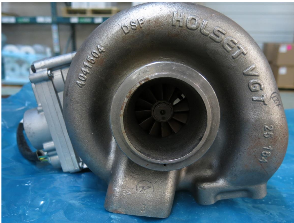
Picture 7: The bottom fan of the turbo engine packaged in VpCI-126 and PE bags after 500 hours. Only small amounts can be seen on the lip where the engine contacted the packaging
