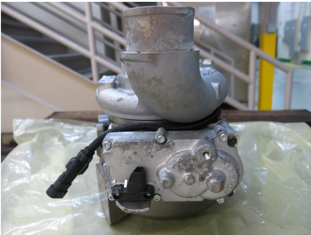
Picture 10: The wire housing of the turbo engine packaged in NT bags after 500 hours. Significant discoloration was observed on the wire housing and surrounding engine body.
