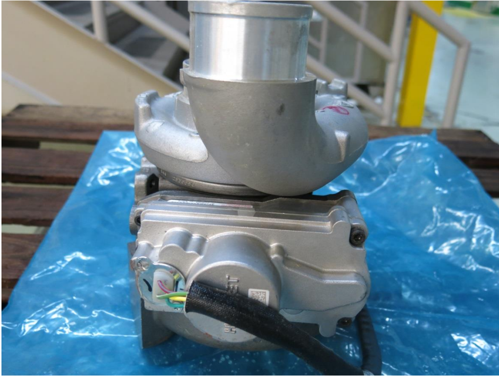
Picture 9: The wire housing of the turbo engine packaged in VpCI-126 and PE bags after 500 hours. No corrosion can be seen on the wire housing or the surrounding body.
