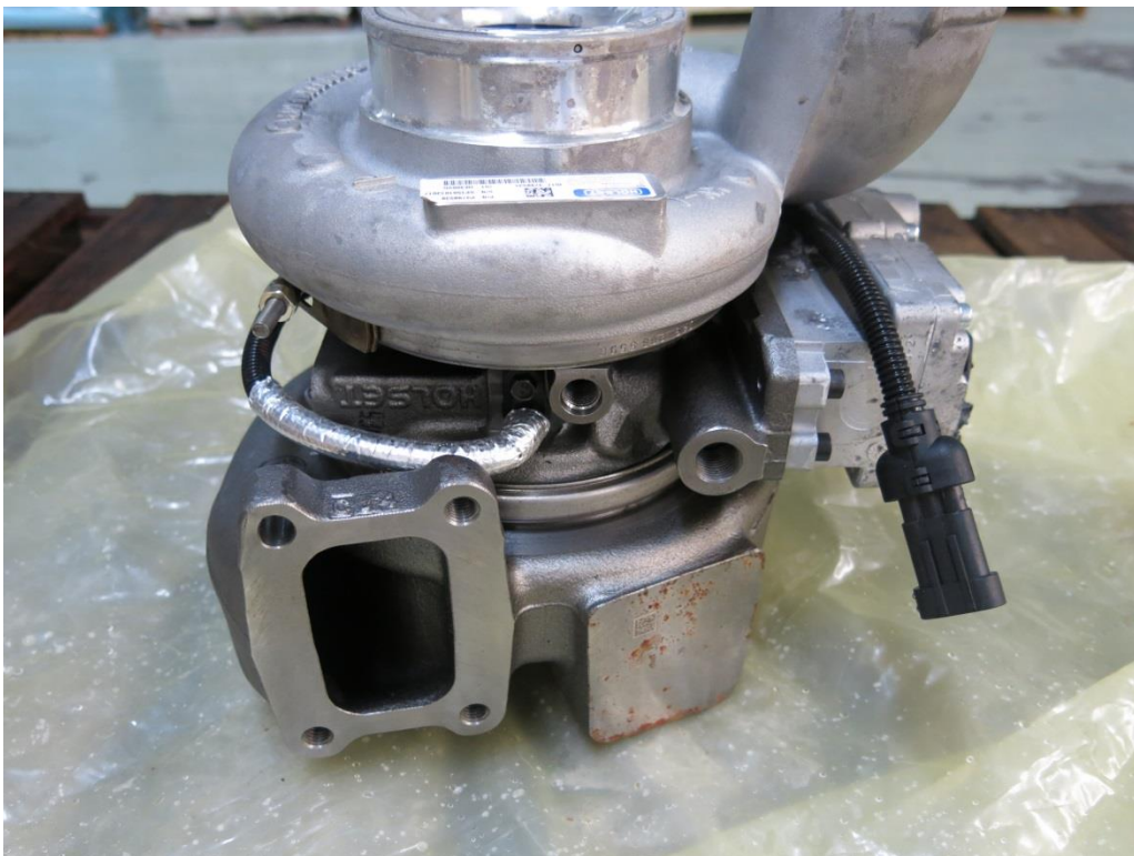
Picture 6: The base of the turbo engine packaged in NT bags after 500 hours. Moderate corrosion can be seen on the flat.
