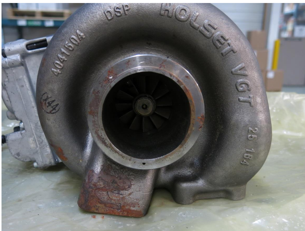
Picture 8: The bottom fan of the turbo engine packaged in NT bags after 500 hours. Severe corrosion can be seen on the lip and body of the engine that sat in contact with the packaging.
