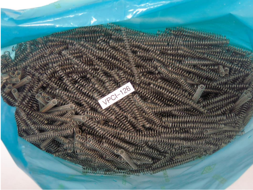
Photo 3: The VpCI-126 bag after 2300 hours of humidity testing
