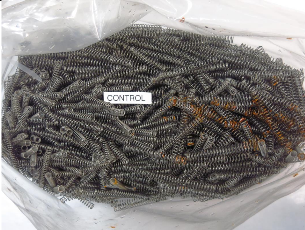
Photo 1: The control bag after 2300 hours of humidity testing
