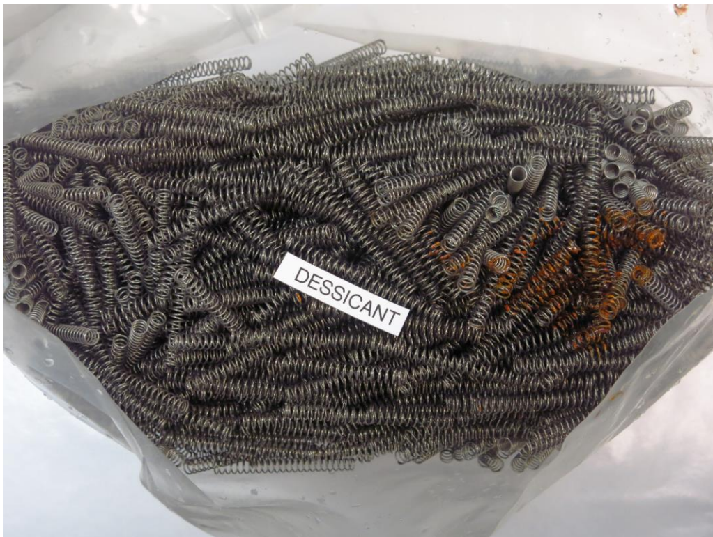
Photo 2: The desiccant bag after 2300 hours of humidity testing. Desiccant was located on the bottom of the bag.
