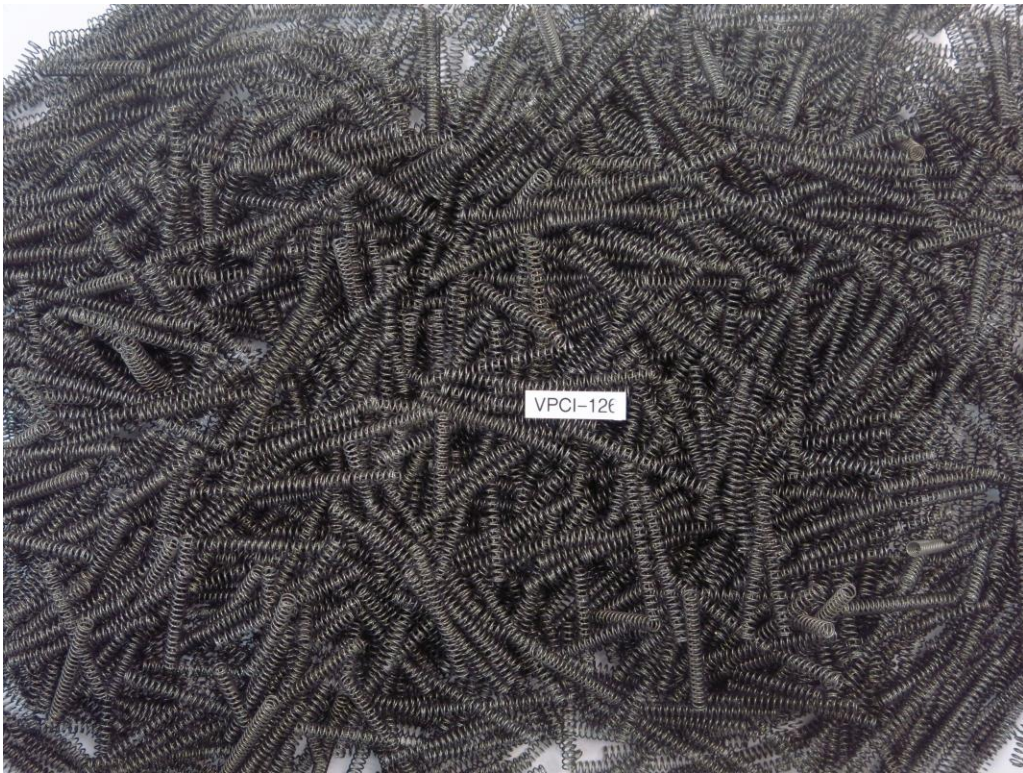
Photo 4: The VpCI-126-protected springs after 2300 hours of humidity testing. Springs were removed from the bag to inspect for any signs of corrosion which may not have been apparent from initial inspection.
