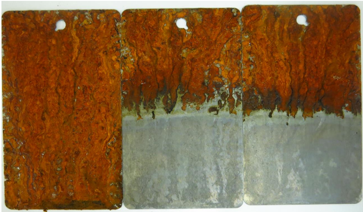
Picture 1: Fully rusted panel compared to 2 panels half cleaned with VpCI-422 and VpCI-415.
