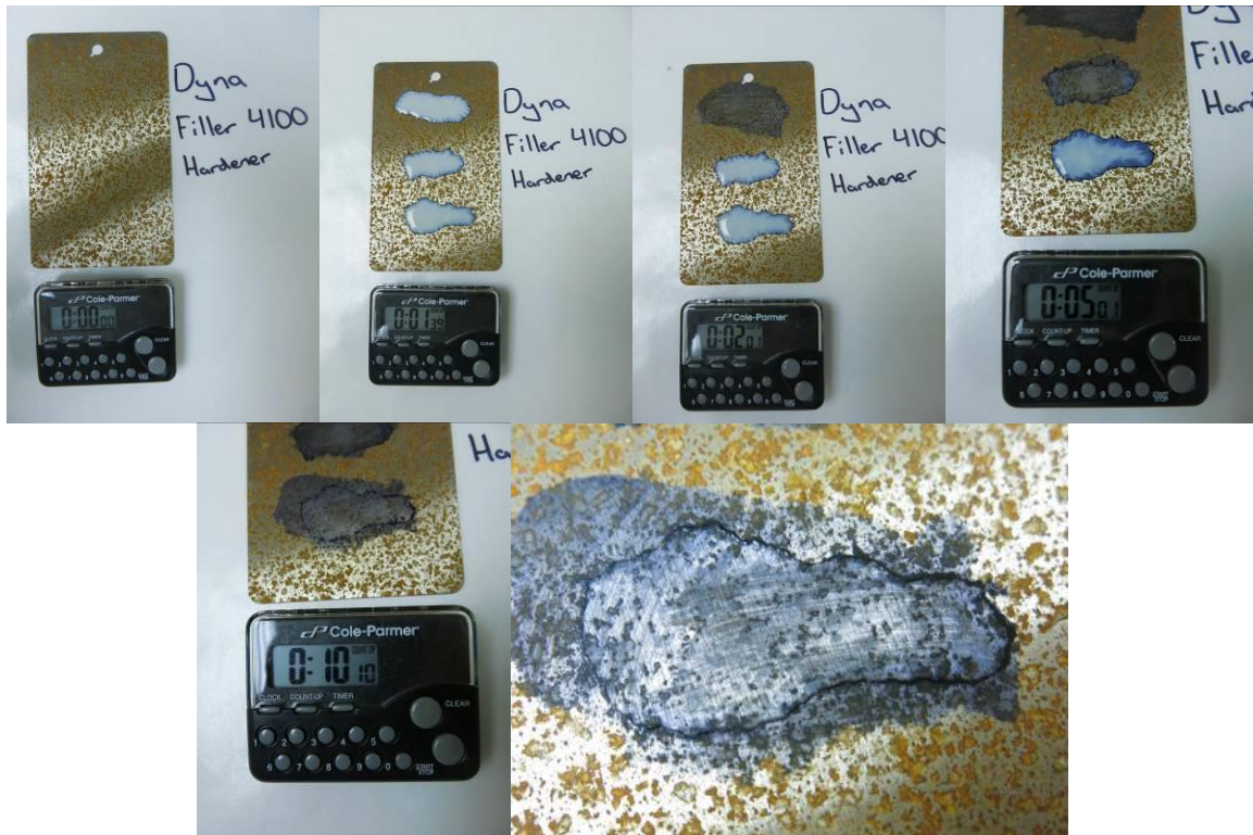
Figure 4: The progression of the DYNA Filler 4100 hardener rust removal testing. Surface still has black oxide even after 10 minutes of cleaning. There is also a ring marking the edge of the product.
