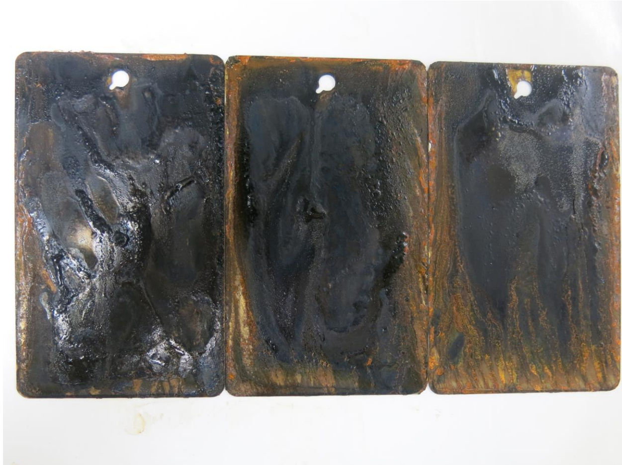
Figure 5: Steel panels coated with DYNA Filler 4100 hardener after 24 hours of exposure to ASTM-B117 conditions.
