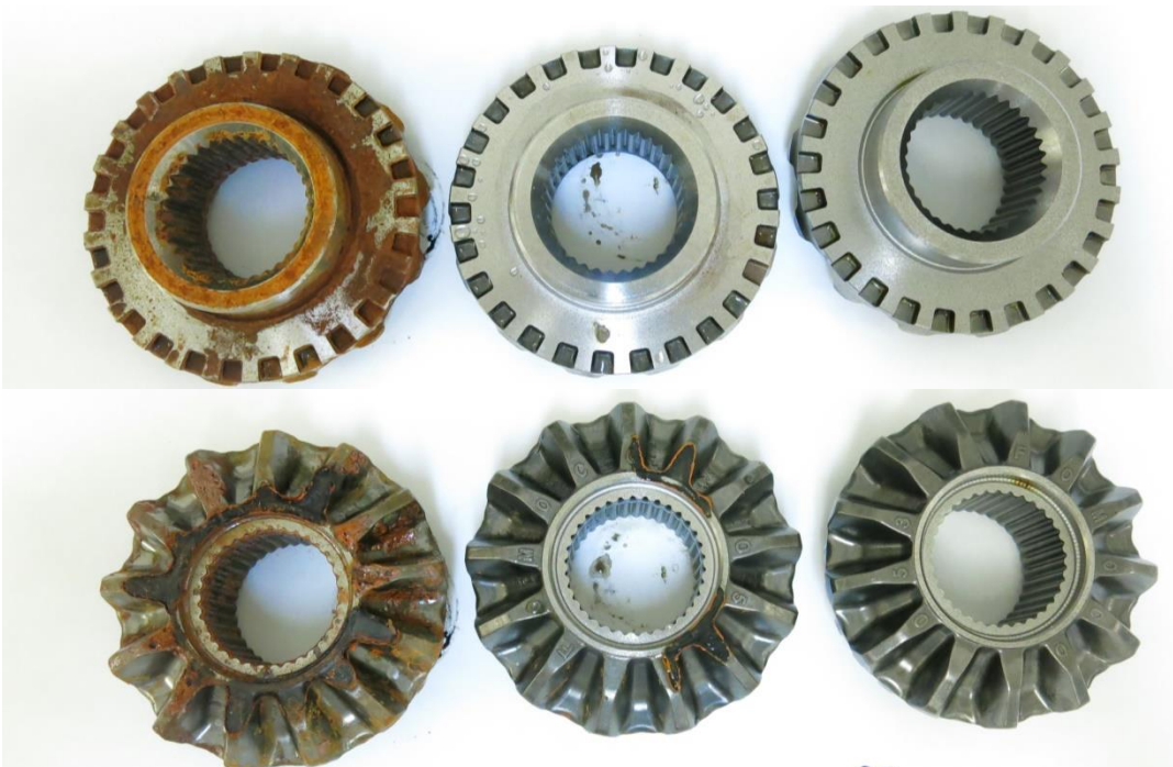
Picture 12: Locking Side Gears – Rust Preventative, from left to right: Compound RP-99S, BioCorr, BioCorr + VpCI-126 bags + VpCI-146 paper.
