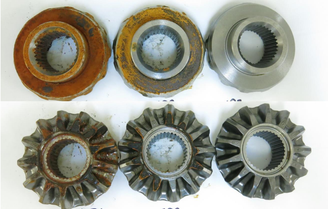
Picture 9: Side Gears – Rust Preventative, from left to right: Compound RP-99S, BioCorr, BioCorr + VpCI-126 bags + VpCI-146 paper.
