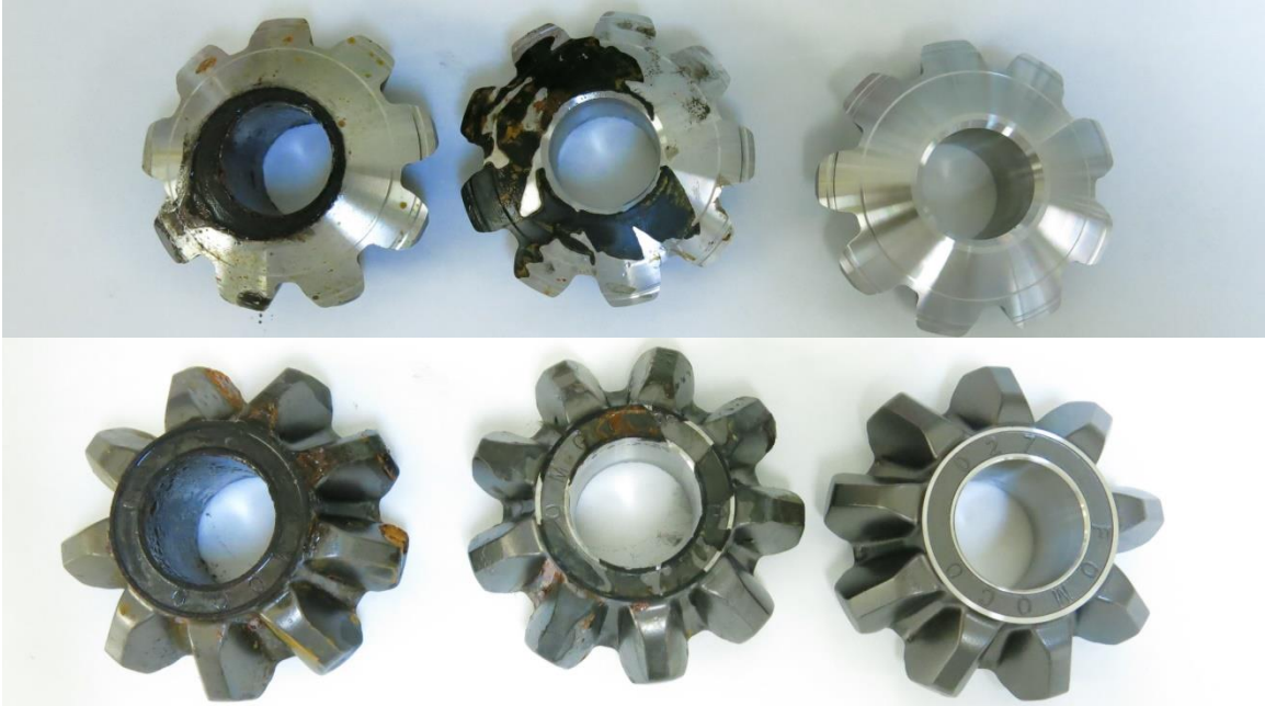
Picture 13: Pinions – Turned, from left to right: Control, ZeRust Paper, Cortec VpCI-126 film + VpCI-146 paper.
