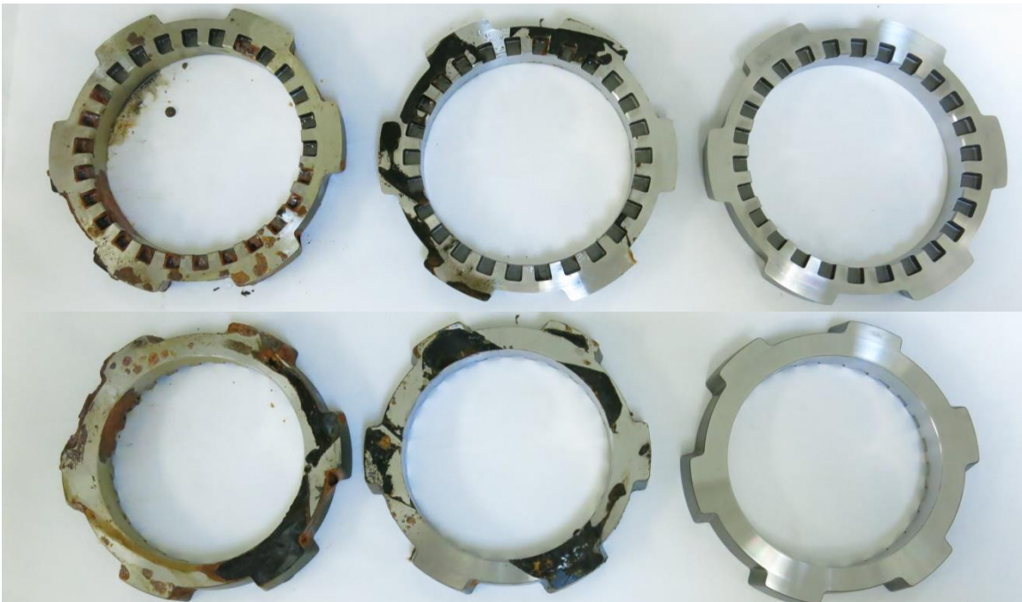
Picture 4: Small Locking Plates – Turned, from left to right: Control, ZeRust Paper, Cortec VpCI-126 film + VpCI-146 paper.
