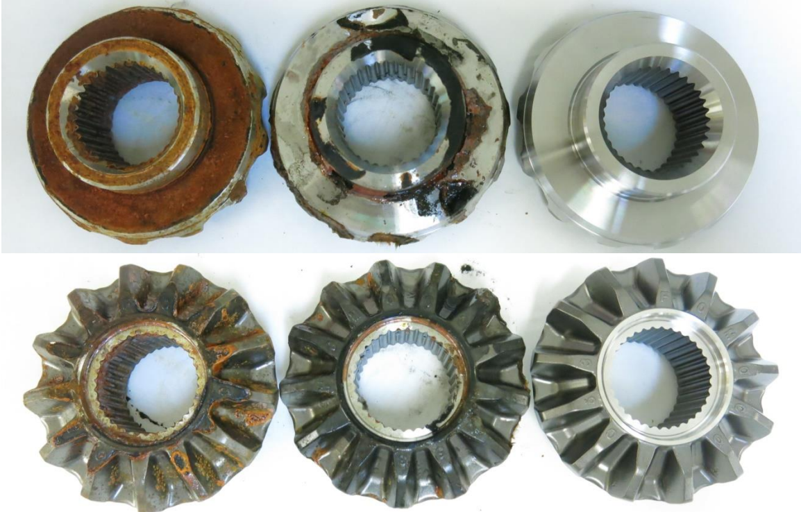
Picture 7: Side Gears – Turned, from left to right: Control, ZeRust Paper, Cortec VpCI-126 film + VpCI-146 paper.
