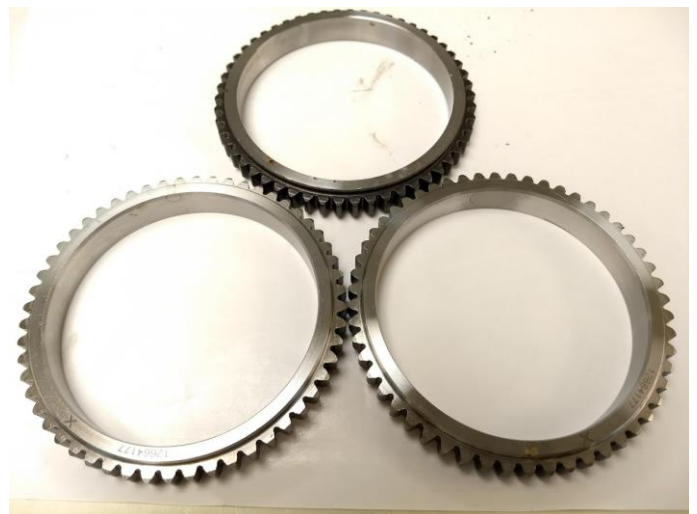
Figure 8. VpCI-325 after 360 hours
