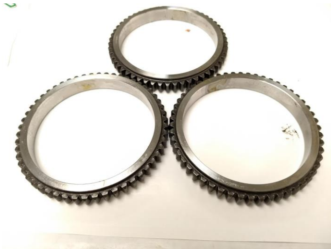
Figure 7. VpCI-329 after 360 hours
