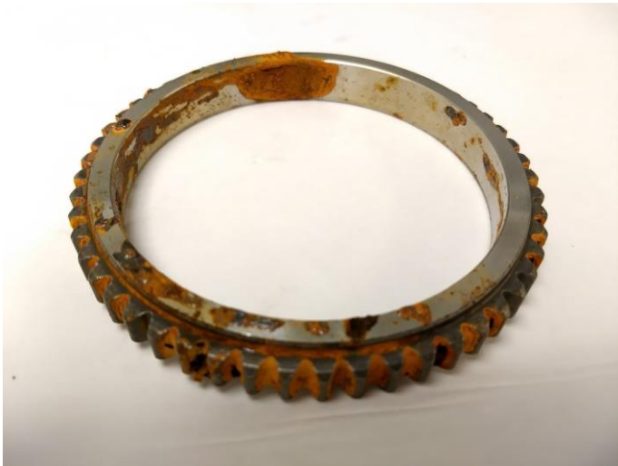
Figure 3. Control after 360 hours
