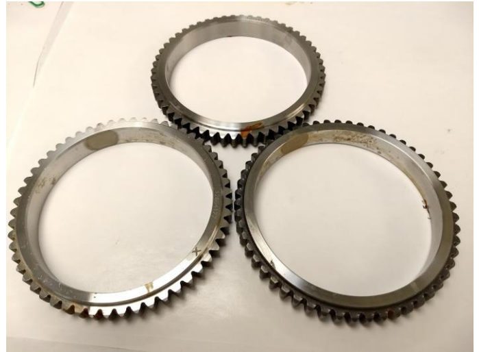
Figure 6. BioCorr ATF after 360 hours
