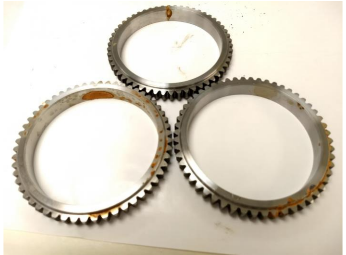
Figure 4. Castrol oil after 360 hours
