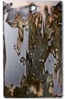
Unprotected mild steel panel
