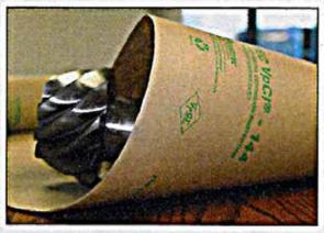
VpCI-144 is an environmentally safe replacement for polyethylene and wax papers, with water vapor barrier properties that are compárable to polyeth-
