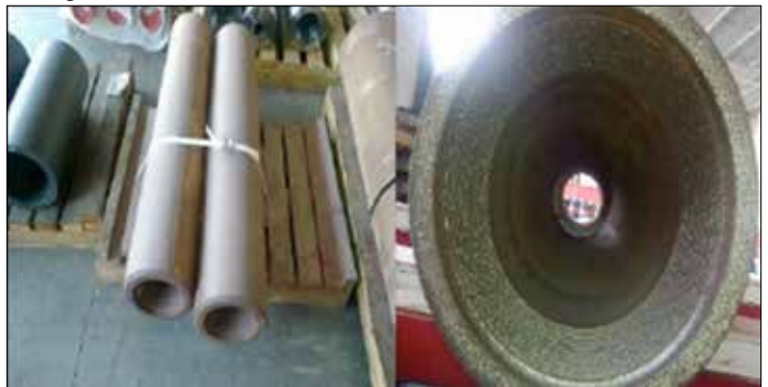
Drilling Tools After Rust Removal using VpCI®
