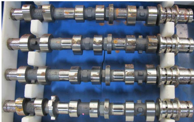
Control after 192 hours of testing according to ASTM D 1748
