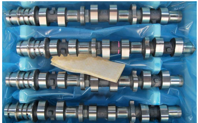
Camshafts protected with BioPad ® after 192 hours of testing according to ASTM D 1748
