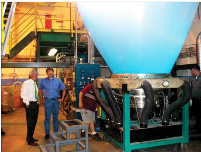
Cortec® CEO, Boris Miksic, FNACE and Tim Bliss, CAF Production Manager monitoring extrusion of VpCI®-126 Blue Film
