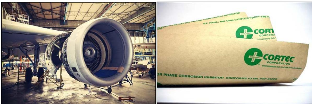
**VpCI® 146 was used for preservation of Indian Navy's Naval Aircraft Engine. After inserting Cortec's VpCI®132 Foam Pads, the entire engine was wrapped with VpCI®146 paper and sealed. By switching to Cortec's method, the navy saved 60 - 70% on current costs and gained a non-hazardous, environmentally friendly solution for long term storage.**
