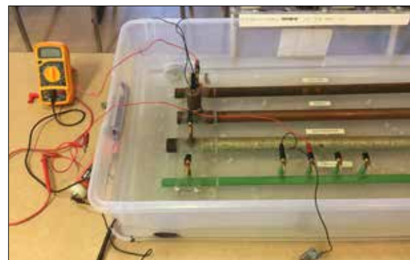
One of the hands-on lab test stations at the corrosion short course demonstrated how different types of metal require different levels of cathodic protection (e.g., bare pipe vs. coated pipe). The strength of the electrical current can be measured by an amp meter.
