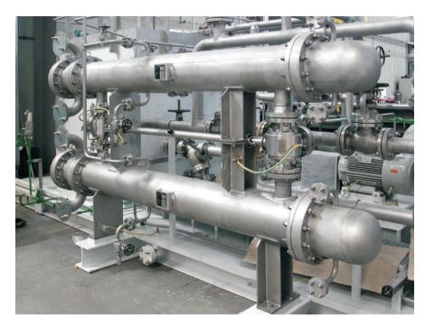
expensive stainless steel to make oil coolers that would resist corrosion. However, the manufacturer wondered if a high-temperature protective coating from Cortec\* would allow them to make carbon steel oil coolers that would resist corrosion as well.
