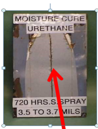
Without VpCIs (more blistering/corrosion)
