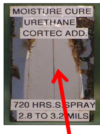
With VpCIs (less blistering/corrosion)
