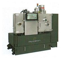
dense aluminum oxide (Al2O3) coatings on heat-sensitive substrates in various industrial metallization applications including off-highway and agricultural equipment engines. Porous Al2O3 layers are used as filters and electrical insulation layers, while dense Al2O3 is used as a barrier and a transmittable optical coating. The USPLD process offers precise micro-
