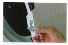
it protects painted surfaces from rocks, gravel, salt, oils, magnesium chloride, and insect and bird wastes. The film is available in rolls of varying widths and lengths, pre-cut in various patterns; improved elongation, memory, and flexibility enable single-piece installations. Suitable applications include hoods, headlamps, fenders, rocker panels, door edges, and mirrors.
