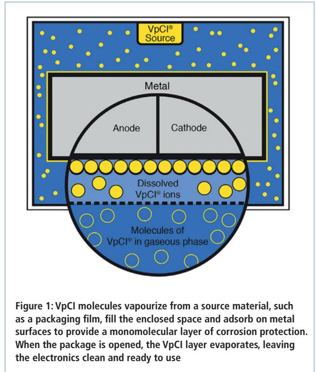
**Figure 1:** VpCI molecules vapourize from a source material, such as a packaging film, fill the enclosed space and adsorb on metal surfaces to provide a monomolecular layer of corrosion protection. When the package is opened, the VpCI layer evaporates, leaving the electronics clean and ready to use
