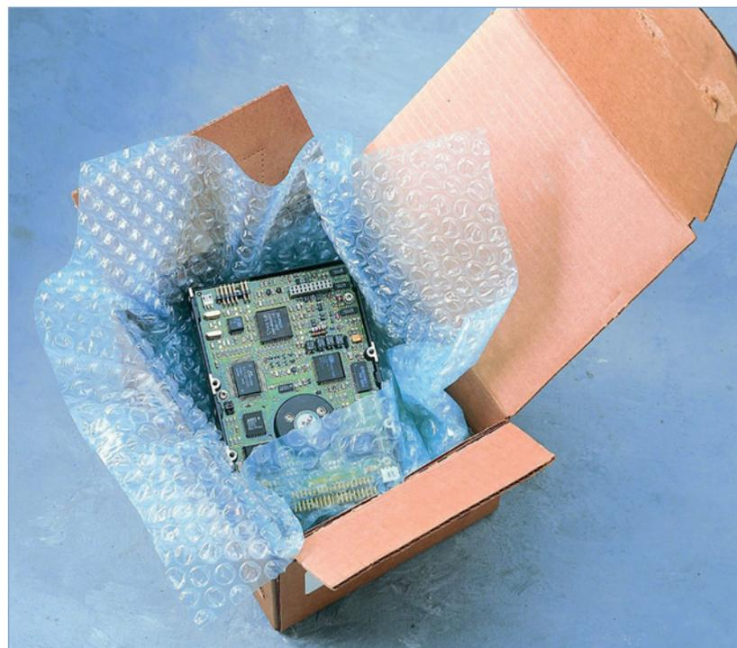
**Figure 3: VpCI technology can be combined with ESD properties in the form of bubble wrap to provide cushioning, and ESD and corrosion protection for sensitive electronics**
