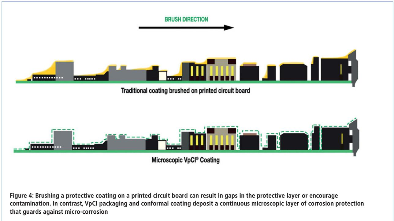
Figure 4: Brushing a protective coating on a printed circuit board can result in gaps in the protective layer or encourage contamination. In contrast, VpCI packaging and conformal coating deposit a continuous microscopic layer of corrosion protection that guards against micro-corrosion
