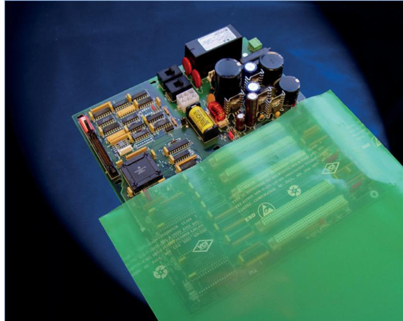
Figure 2: The use of ESD VpCI film is an excellent strategy for reducing corrosion claims and reducing packaging labour and material costs
