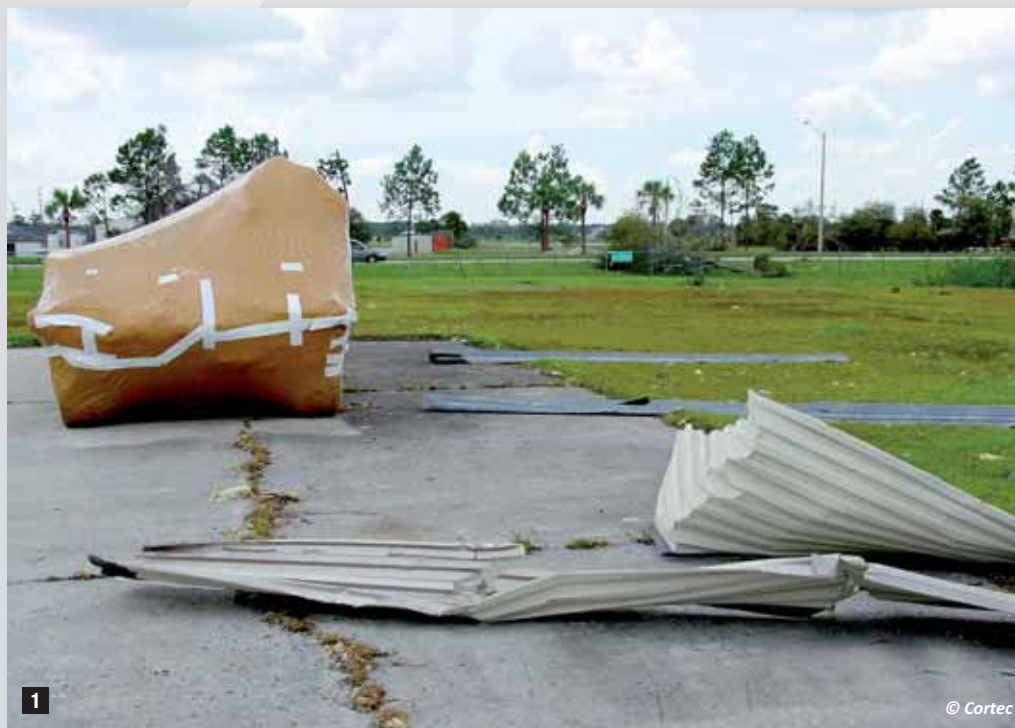
1 The packaging has been created by MilCorr® VpCI® Shrink Film. After exposition to hurricane's power, this film demonstrated that is able to resist to any type of storm.
