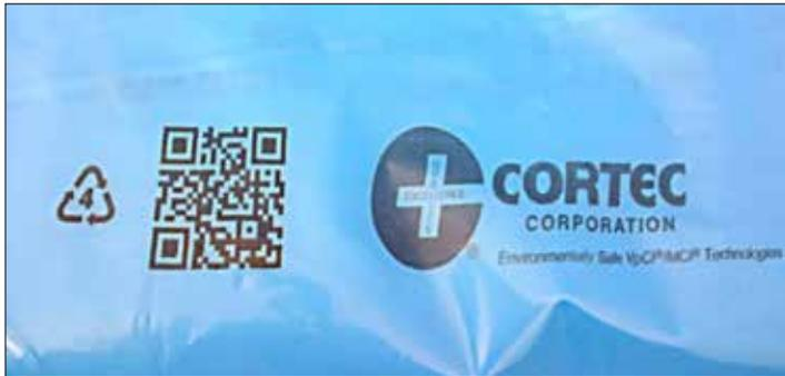
The VpCI® film that is produced on line E19 now displays both the Cortec® logo and QR code for instant brand recognition. Anyone who scans the QR code with a smart phone will be taken directly to Cortec's website to learn more about Cortec's innovative products. The new printer also allows greater flexibility on what can be printed and does not require a separate print plate for each project. The results are cost reduction and increasing opportunities for printing customization.
